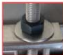
Nuts are coated with molybdene to prevent galling
